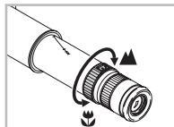
The focusing will be done by turning the adjustment ring for focusing.
