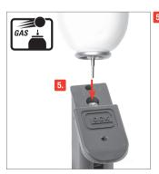
5. Keep the magazine with gas tank tilted.
