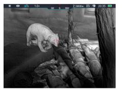
hold the **M** (7) +**Down** (8) buttons at the same time to turn the hotspot tracking function on/off.
