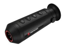
HIKMICRO LYNX S LE10S thermal monocular is equipped with a  $256 \times 192$  infrared detector and an  $800 \times 600$  OLED display. It supports functions of observation, distance measurement, hotspot, and so on. The high-sensitivity built-in thermal detector provides you with a clear view even in total darkness. The monocular is mainly applied to scenarios such as hunting, hiking, searching and rescuing, etc.
