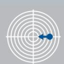
To move the point of impact **leftward** – turn the horizontal adjustment knob away from the 'R' arrow.
