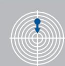
To move the point of impact **down** – turn the vertical adjustment knob in the opposite direction to the 'UP' direction.
